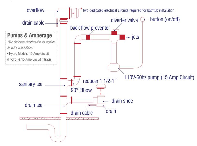
We have taken responsible precautions to ensure the Auto Drain is suitable for residential plumbing. It is the responsibility of the installer to insure the sanitary system is acceptable for the use of the Auto Drain. We do not accept responsibility for damage arising from the use of the Auto Drain.\*
